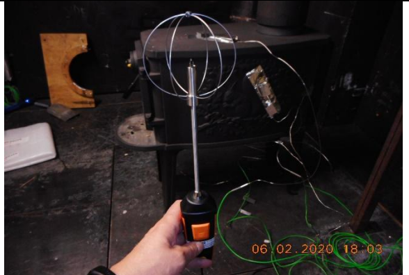
12) Measurement of air velocity at the end of the Medium fire test
