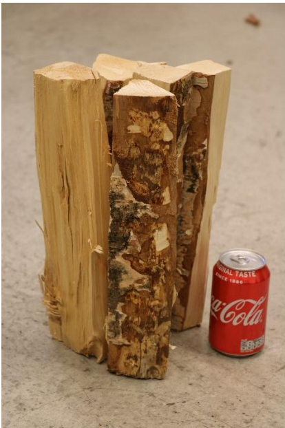
High Fire Load sample Nominal length 13''
