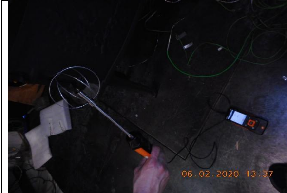
11) Measurement of air velocity at the beginning of the Medium fire test
