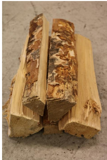
High Fire Load sample Arrangement
