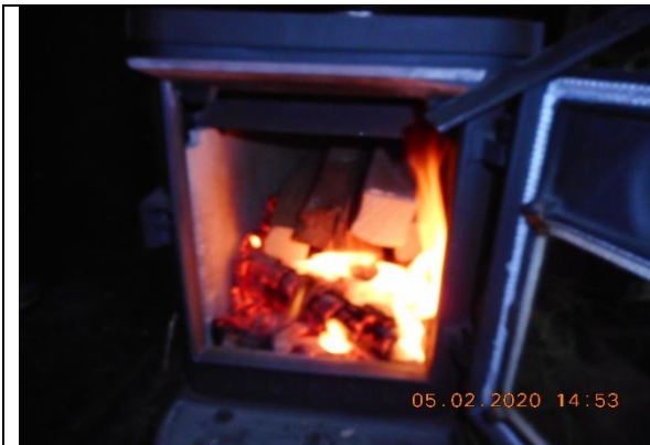
17) Firebed after loading of the LF fuel batch
