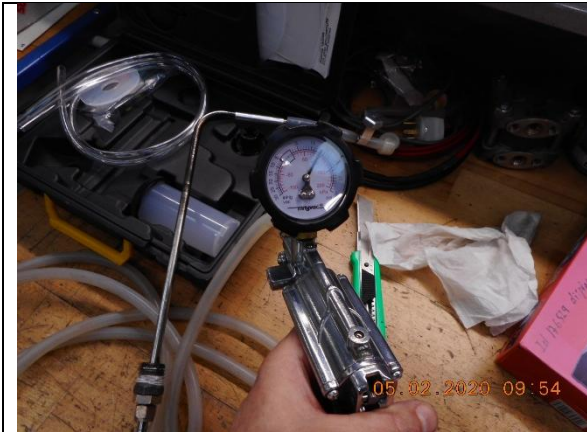
1) Leakage check of pitot tube
