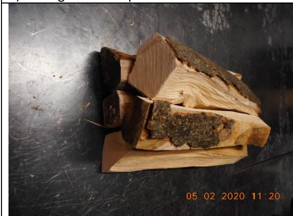
3) High fire fuel load of 5 logs of beech wood
