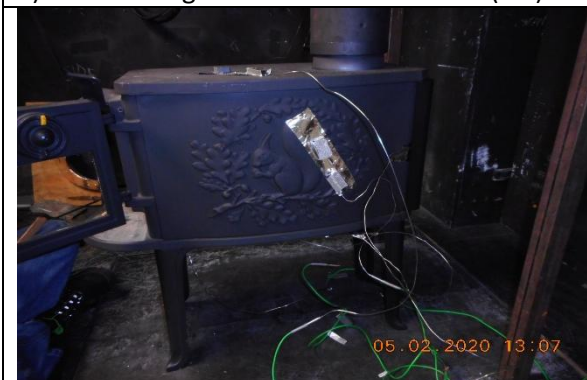
7) Morsø 2B with surface temp TC on test rig
