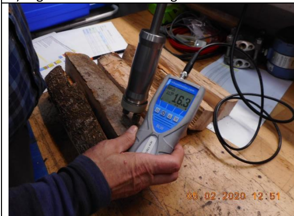
5) Check of High fire load fuel moisture (wb)
