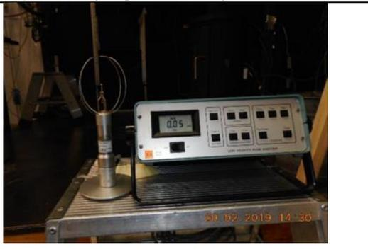
14) Repeated measurement of air velocity
