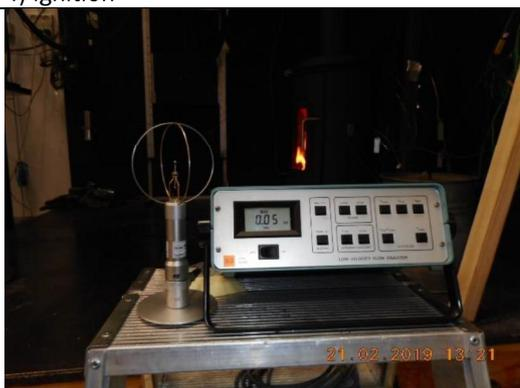
6) Measurement of air velocity
