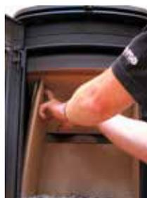
2. Tip the side bricks and remove them from the fire chamber.
