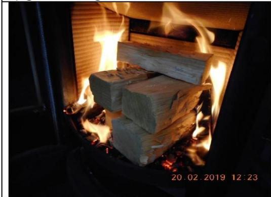
11) 5 min after loading of the MF fuel load
