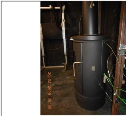
1) 6100B stove on test rig with surface TCs
