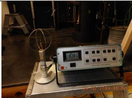
7) Measurement of air velocity
