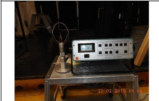
15) Final measurement of air velocity
