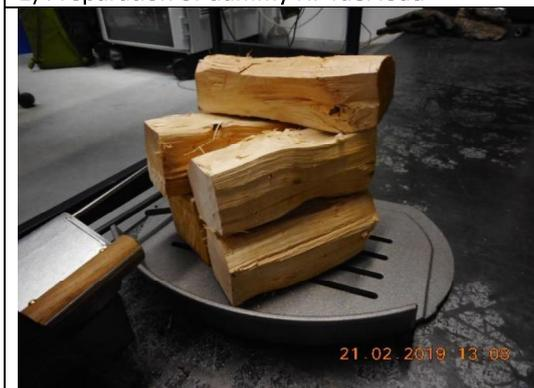
3) Arrangement of dummy HF load
