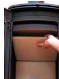
5. The upper baffle is removed from the brackets and lifted out of the fire chamber.
