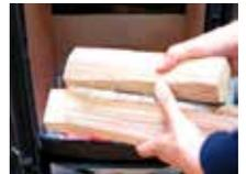
8. Close the door. Leave the primary air supply fully open. If it does not light, leave the door slightly ajar to allow the necessary amount of air in to ignite the wood. Close the door again once the wood has kindled.
