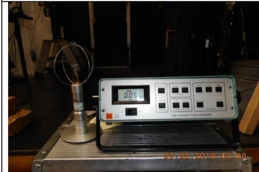
13) Measurement of air velocity
