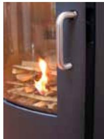
4. After lighting, partially close the door, leaving it open an inch or two to allow in plenty of combustion air.
