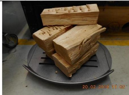
8) Arrangement of the HF fuel load
