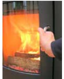
9. After a few minutes, adjust the primary air supply to suit your heating requirements. Make sure that there is always enough air to sustain clear, enduring flames when you reduce the amount of combustion air, and afterwards.
